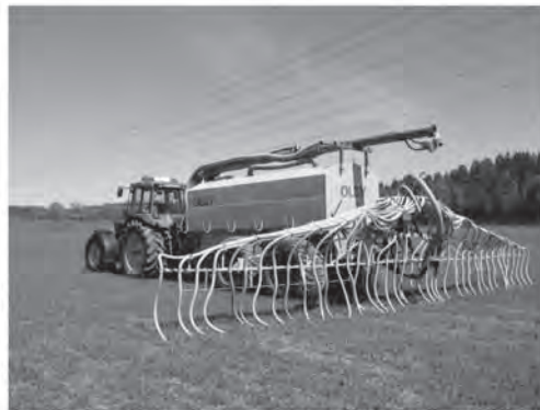
Figure 1.4 Conventional slurry spreader used for application of urine
