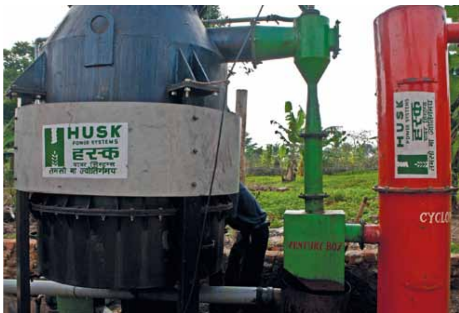
Figure 10.12 Iiribogo gasification project utilising corn husks and sawdust, located in Muduuma Sub-county, Mpigi District, Uganda (photo: Linda Strande).
